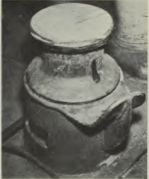
Figure 7-9.—Roller bitt saves line.
